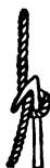
FIG. 39.—Proper way to make first "hitch" of rope on hook of counterweight.
